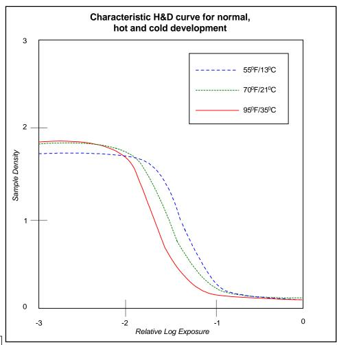
At 71° F/21° C: D-Max = 1.70 D-Min = .10 Slope = 1.65
