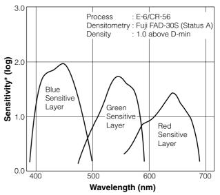
Sensitivity equals the reciprocal of the exposure (J/cm²) required to produce a specified density.
