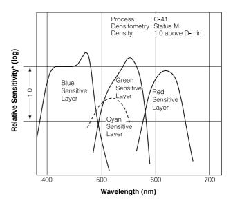
Sensitivity equals the reciprocal of the exposure (J/cm²) required to produce a specified density.
