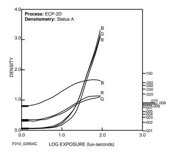
To find the rms Granularity value for a given density, find the density on the left vertical scale and follow horizontally to the characteristic curve and then go vertically (up or down) to the granularity curve. At that point, follow horizontally to the Granularity Sigma D scale on the right. Read the number and multiply by 1000 for the rms value.
