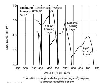
These curves depict the sensitivity of this film to the spectrum of light. They are useful for determining, modifying, and optimizing exposure for blue- and green-screen visual effects work.
