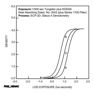
The curves describe this film's response to red, green, and blue light. Sensitometric curves determine the change in density on the film for a given change in log exposure.<sup>3</sup>
