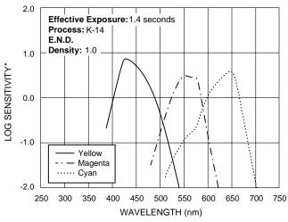
\*Sensitivity = reciprocal of exposure (erg/cm<sup>2</sup>) required to produce specified density
