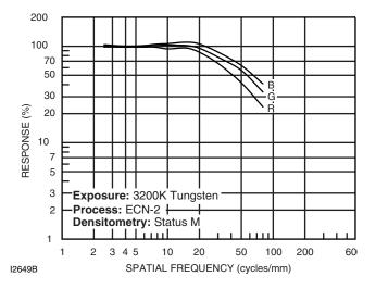
This graph shows a measure of the visual sharpness of this film. The x-axis, "Spatial Frequency," refers to the number of sine waves per millimeter that can be resolved. The y-axis, "Response," corresponds to film sharpness. The longer and flatter the line, the more sine waves per millimeter that can be resolved with a high degree of sharpness—and, the sharper the film.
