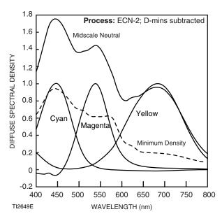
These curves depict the spectral absorptions of the dyes formed when the film is processed. They are useful for adjusting or optimizing any device that scans or prints the film.
