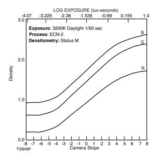
The curves describe this film's response to red, green, and blue light. Sensitometric curves determine the change in density on the film for a given change in log exposure.<sup>4</sup>
