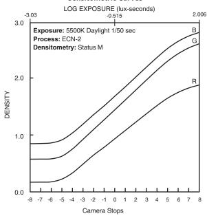
**Note:** The exposure scale for VISION3 5203 / 7203 Film is longer than previous VISION and VISON2 Films. Because of the extended highlight latitude we have expanded the exposure scale from a 0-4 increment to a 0-5 scale. In addition to the longer exposure scale, we are plotting 21 steps instead of 20.
