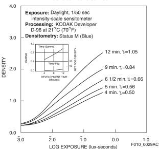
$<sup>^\</sup>dagger$  Develop to recommended control gamma of 0.65 to 0.70 calculated using Status M densitometry (blue)..
