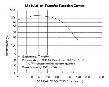
This graph shows a measure of the visual sharpness of this film. The x-axis, "Spatial Frequency," refers to the number of sine waves per millimeter that can be resolved. The y-axis, "Response," corresponds to film sharpness. The longer and flatter the line, the more sine waves per millimeter that can be resolved with a high degree of sharpness—and, the sharper the film.
